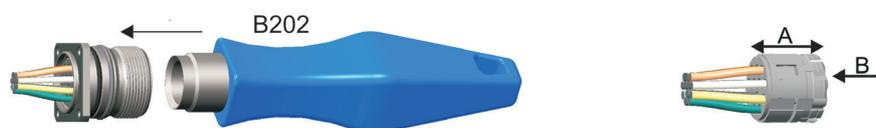
After assembly the connector has to be checked for the functions of the safety precautions (according to EN 60204-1, VDE 0113 Teil 1)
