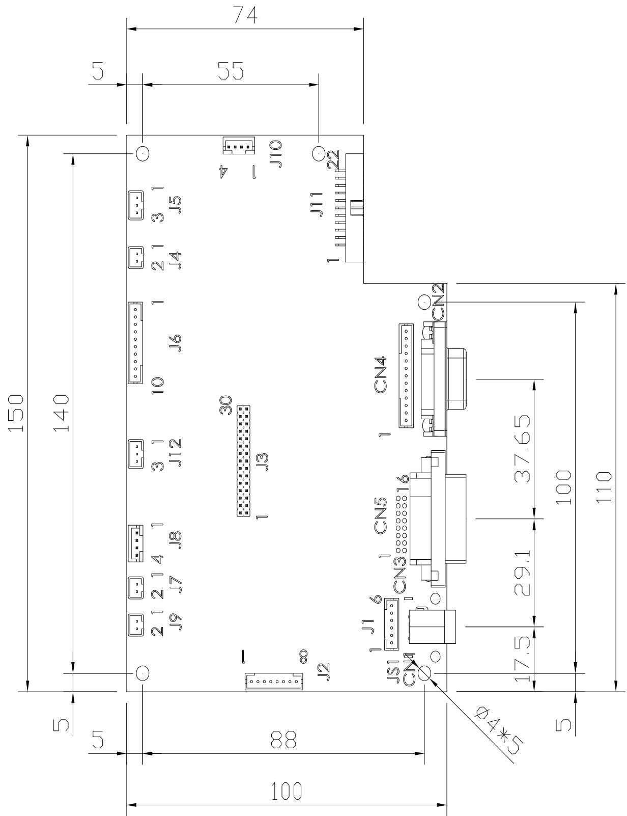
I/O BOARD 160mmX25mmX15mm
