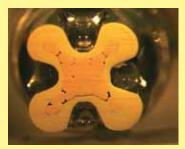
Crimp-cross section HARTING crimp profile
